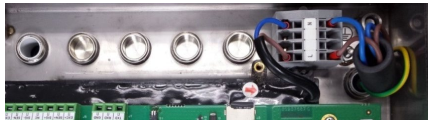
Figure 2-4: AC Power Input Connector, Cover Removed
