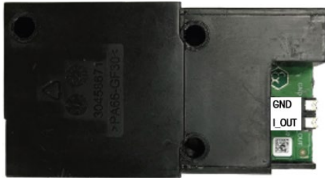
Figure 2-14: Intrinsically Safe Analog Output Option Board
