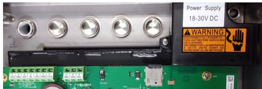
Figure 2-5: DC Power input Connector with Cover
