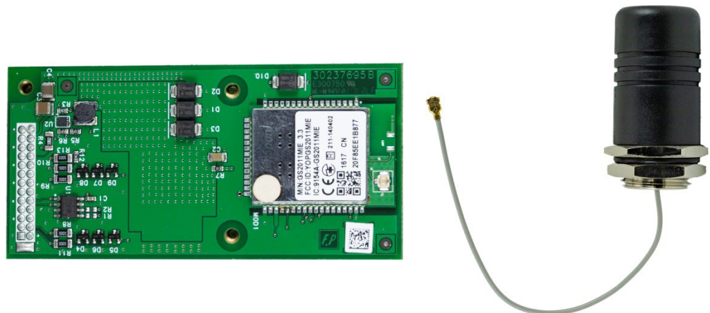
Figure 2-16: IND256x WiFi Option Board and Antenna
