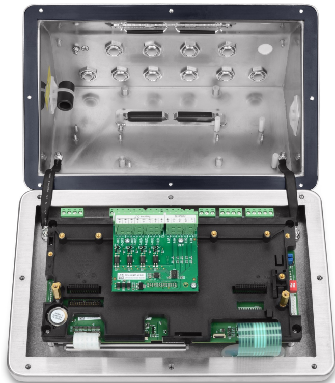
Figura 32: Interface de E/S discretas, instalada
