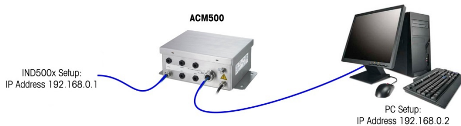
Figure 72: Example: IP Address Configuration (Crossover or Hub Configuration)
