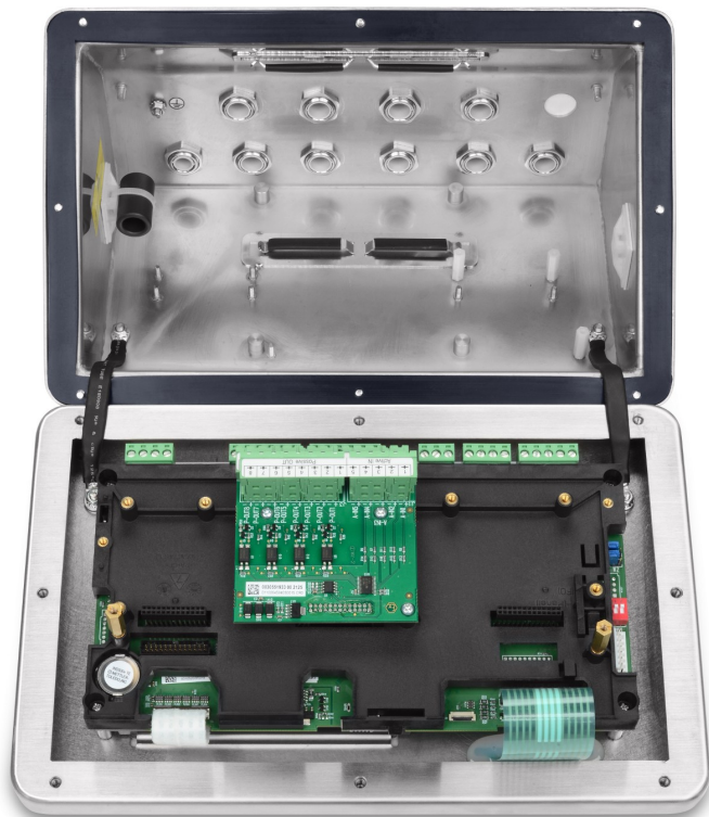
Figure 32: Discrete IO Interface, installed
