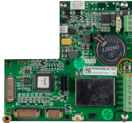
Figure 3-2: Setup Switch Location on Terminal Main Board
